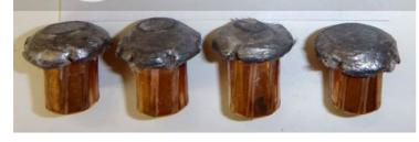
51 Alaskan (.510) 1:15 Twist Rate 350 BBW#13 LG HP Muzzle Velocity 2175 fps 22 Yd Impact Velocity 2070 fps Blades 4-6 Inches X2--18 Inches Total Penetration
