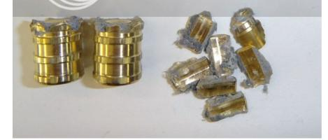
Penetration is nearly identical for both. In animal tissue, the NonCon "Blunt Trauma Base", as it is now termed, will penetrate deeper than the Conventional bullet.
