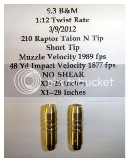
Up the velocity by only around 100 fps and we get perfect shear, and better performance than I expected. At the low end velocity shear point, there is still a good bit of trauma inflicted, more than what I expected, and penetration was good as well.
