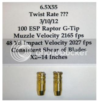
Down at 1862 fps Impact both bullets still sheared, however one was just starting to show signs of instability and not shearing. So, this is as low as I went, and declared that 1900 fps impact is the Low Velocity Shear Point for this bullet. Below 1900 fps impact I think it starts to get iffy at best as you can see.
