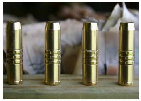
Same boring results as the 470 and 375. The mark on the bullet second from right is from my vice when I pulled the bullet out of the 2 by 6.
