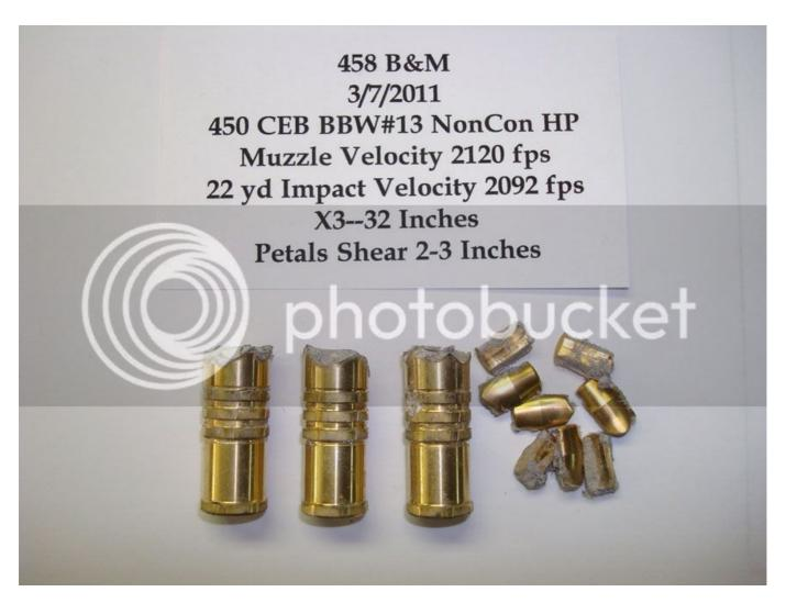
In light of this we have changed the 458s as well, enlarging the cavity, thinning the blades for lower velocity shearing.
