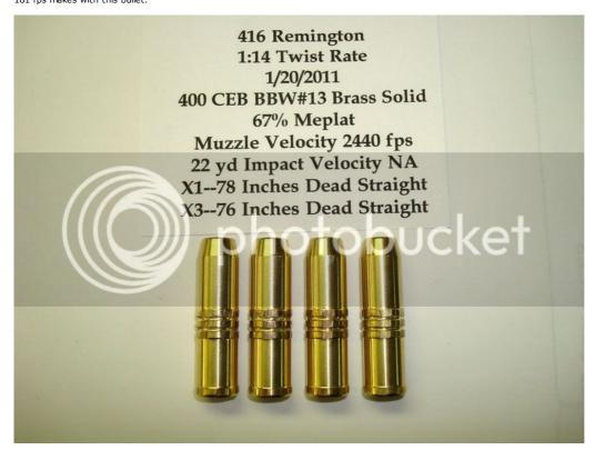
Roughly an 8% increase in velocity gave us roughly an increase of 13% in penetration. It also allowed the bullet to give dead straight penetration as well. Velocity is an important factor to consider, as we already know.
