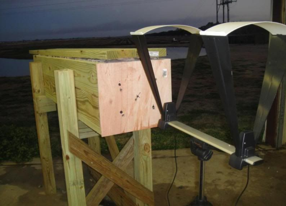
Above is the test box with chronograph.
