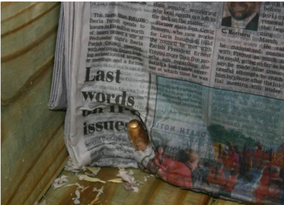
Typical position of Woodleigh bullet found in media.
