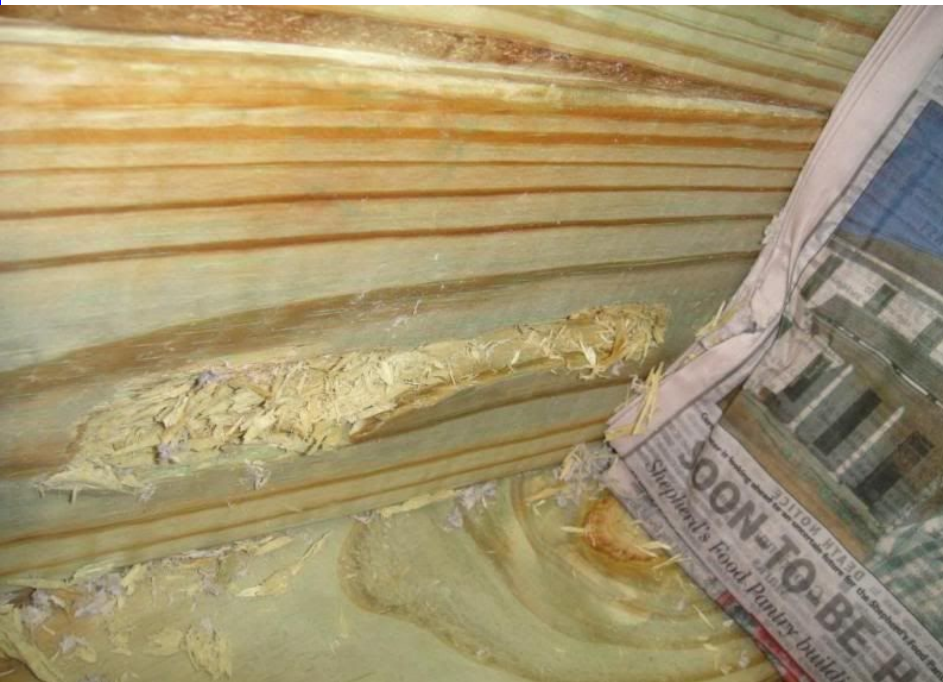
Above is typical damage to the test box caused by the Woodleigh bullets veering off line.
