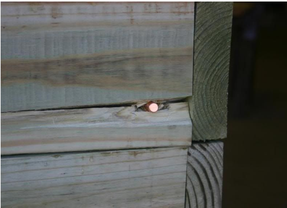
The above picture is taken from outside of box. It is a North Fork bullet after traveling through 72" of test media.
