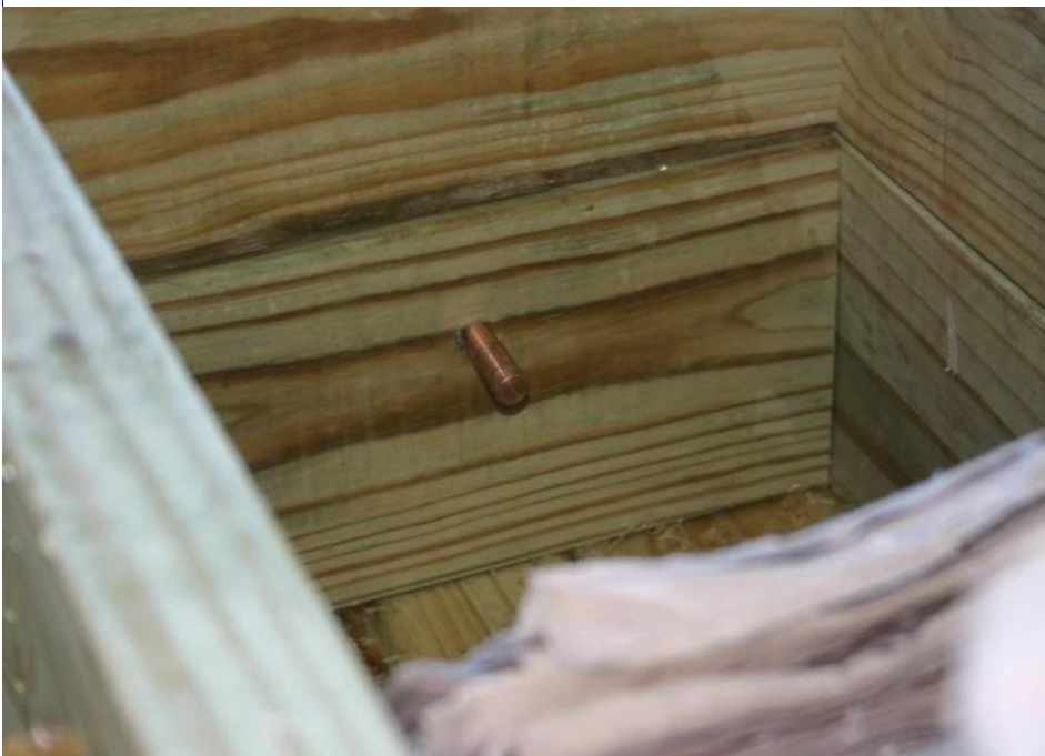
The above picture is taken from inside of box. It is another North Fork bullet after traveling through 72" of test media.
