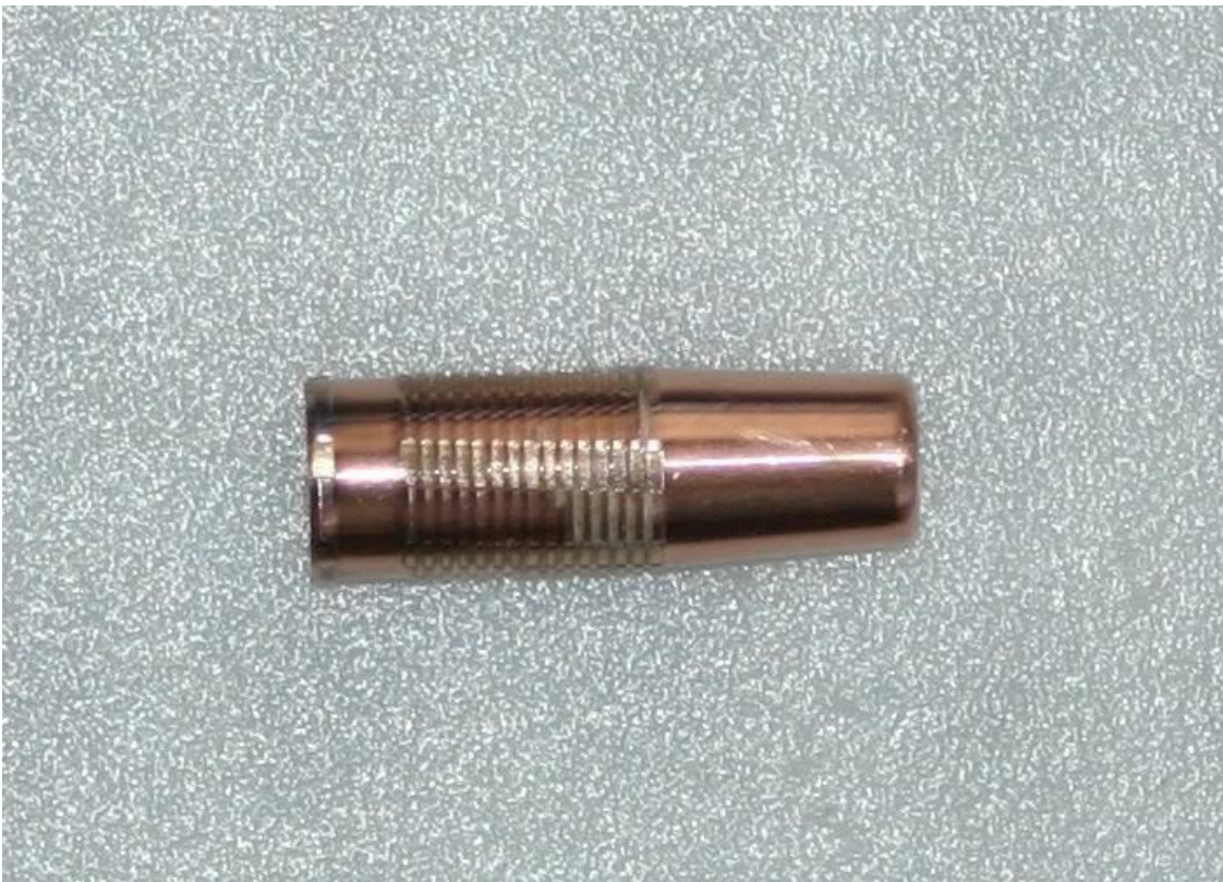
The above picture is of the typical condition of North Fork bullet after firing.
