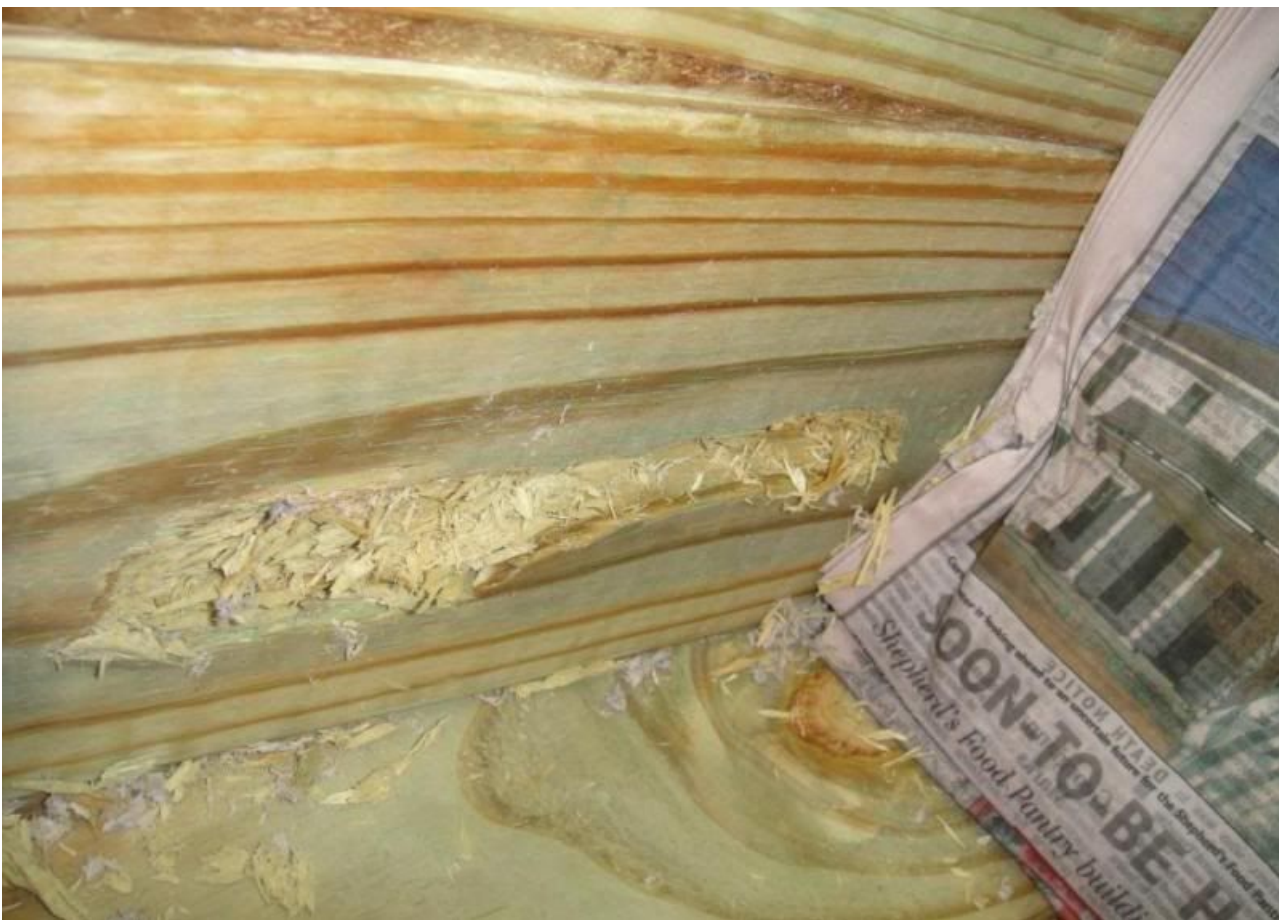
Above is typical damage to the test box caused by the Woodleigh bullets veering off line.
