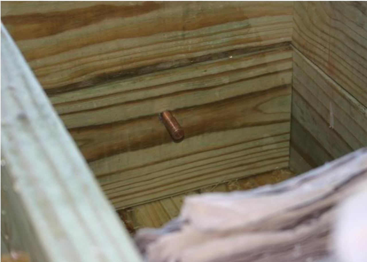
The above picture is taken from inside of box. It is another North Fork bullet after traveling through 72" of test media.
