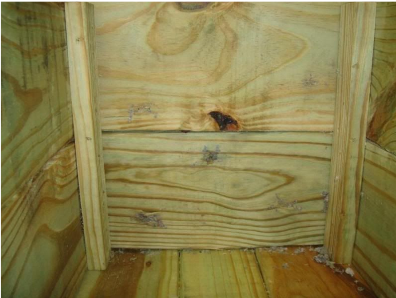
Note the relation of the holes in the bulkhead (set 12" back) and the luan in the picture above. The first 12" was very straight. After hitting the 2 by 6 the bullets went of course.
