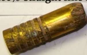
On this Barnes that got the TRex test you see most of the smaller width bands are pretty well wiped, you pick up the engraving on the larger bottom band.
