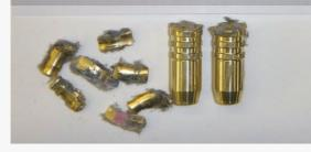
338 Ultra 1:10 Twist Rate ?? 3/5/2012 200 Raptor Solid Muzzle Velocity 3218 fps 48 Yd Impact Velocity 2926 fps Retained--200grs X1--56 Inches X1--58 Inches Cket
