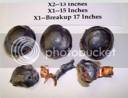
Now what you see is that one of the four broke up. Being smaller across the front, it was able to drive a bit deeper, even though it broke. In our conventional thinking, this would be basically one failure in 4. Or, a 25% failure rate, or 75% success rate, depending on your optimism.
