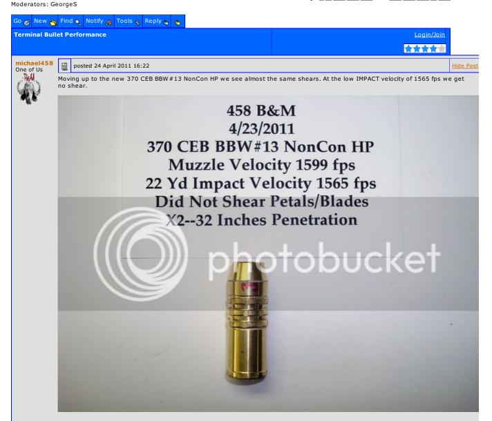
But when we get to an impact velocity of 1665 fps we see that both bullets shear without an issue. I would put low end effective shear at 1650 fps with these.
