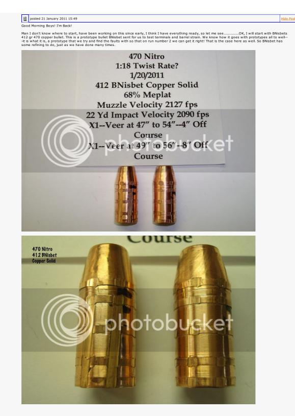
Well right off we see that is not bad performance on terminals for total penetration. Losing stability at 47-49 inches, twist rates could have contributed some to this. Meplat measures 68% so that is a good size, but the edges of the meplat are SHARP---need a radius on there like the BBW #13s.
