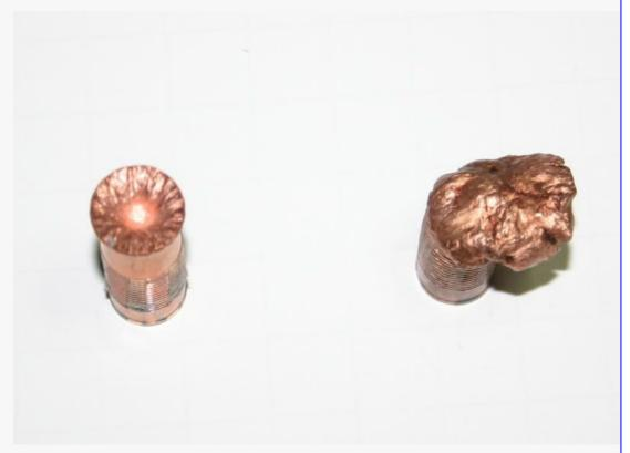
The bullet on the right was the only .474 500 grain North Fork Cup Point I recovered from a buffalo. The bullet on the left was from test media. Muzzle velocity was around 2100 FPS.
