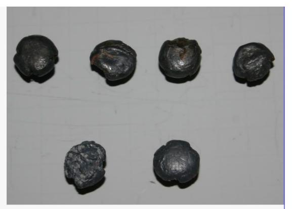
The two above pictures are of 300 Grain North Fork bullets. The top row are bullets removed from a sable, kudu, and wildebeest. The bottom row was from test media (wet newspaper and 2 by 6).
