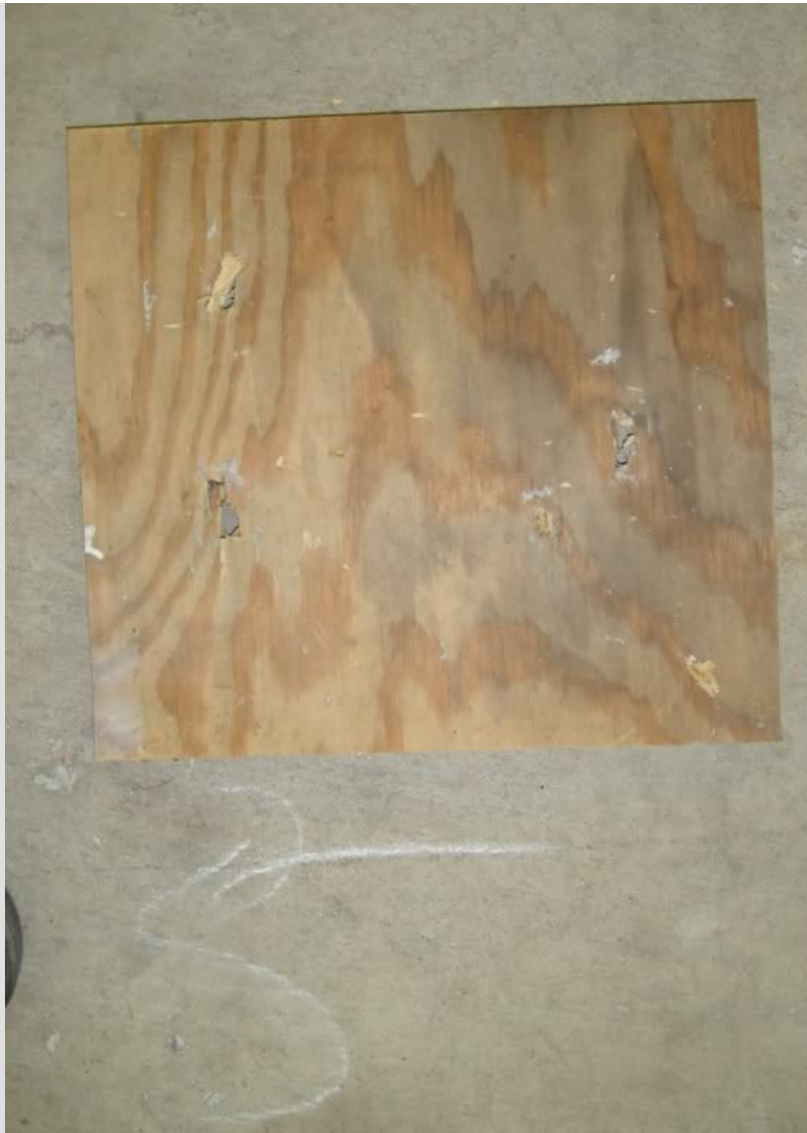
The picture above is the 5th piece of plywood the bullets penetrated. Note the location of the holes as they relate to the first picture. Bullets are beginning to go sideways and off course.
