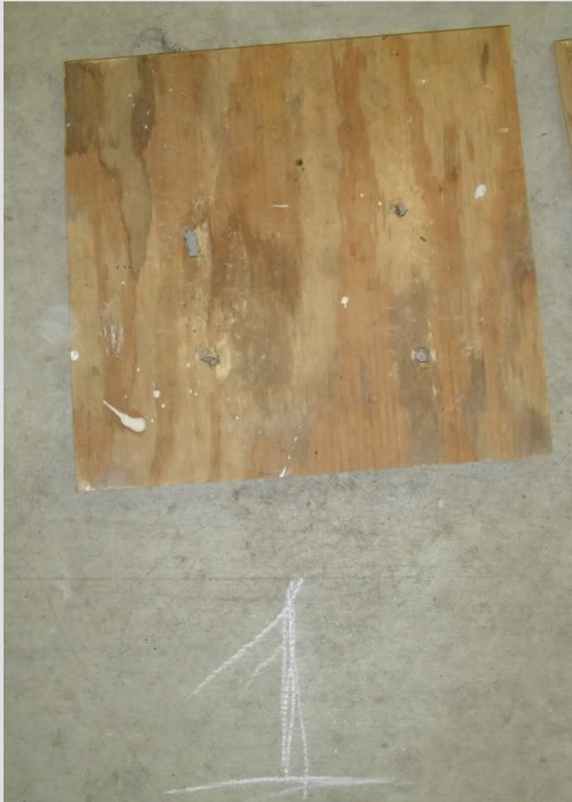
The picture above is the first piece of plywood the bullets penetrated. Note the location of the holes.
