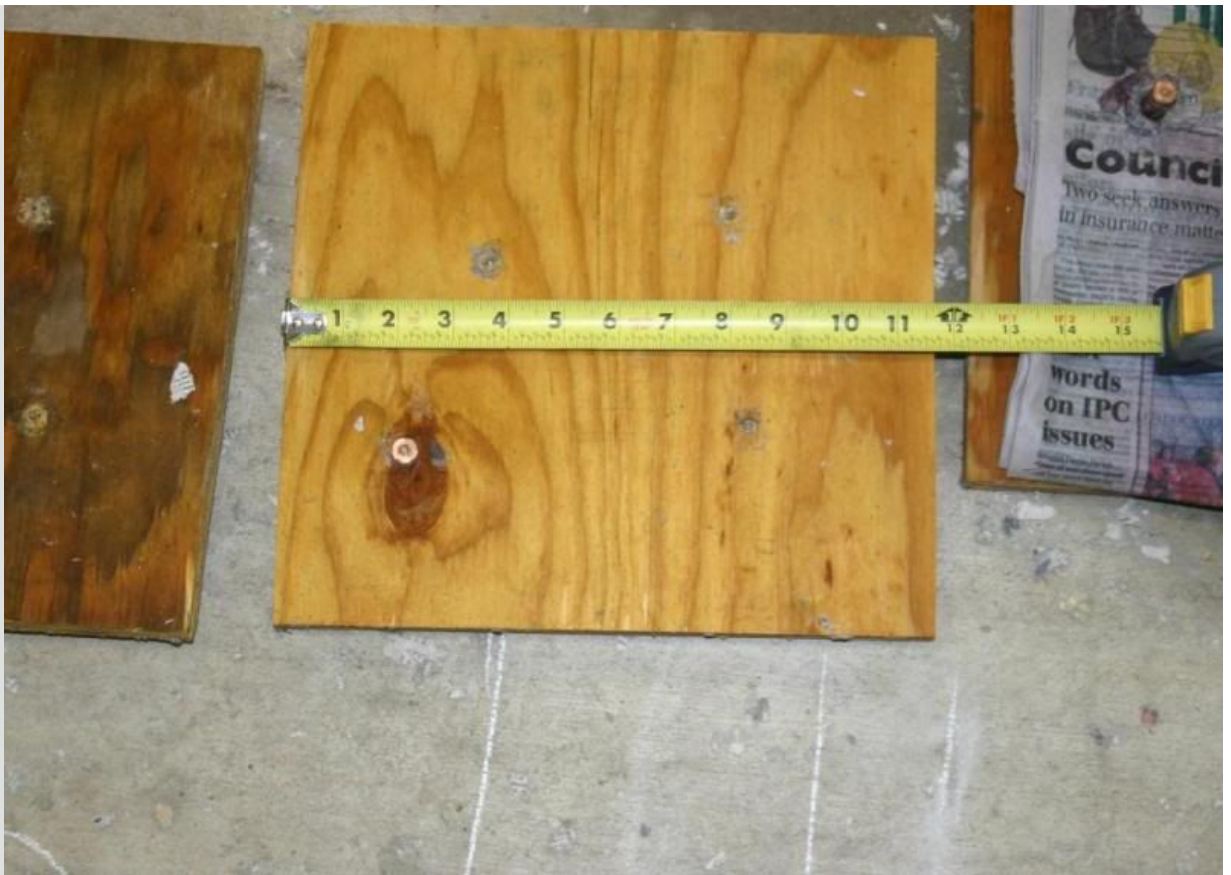
The picture above is the 11th piece of plywood the bullets penetrated. Note the location of the holes as they relate to the first picture.
