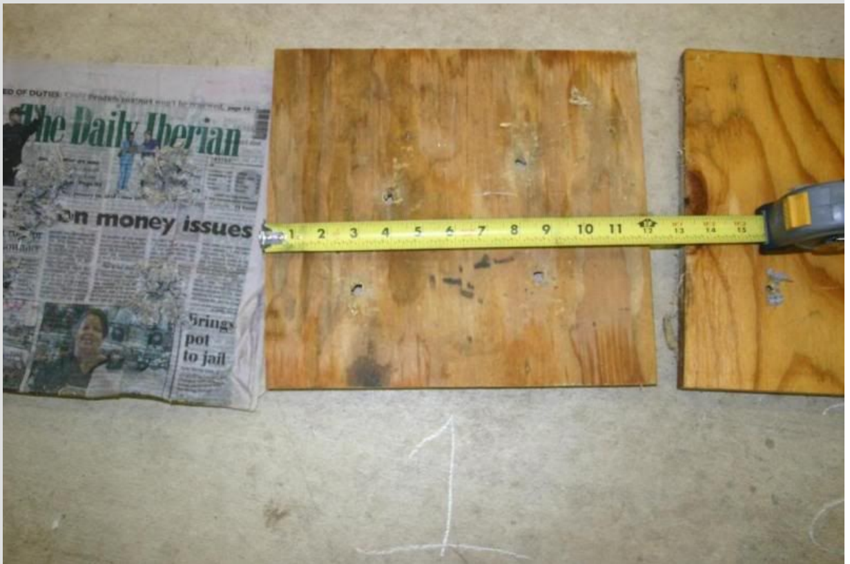
The picture above is the first piece of plywood the bullets penetrated. Note the location of the holes.
