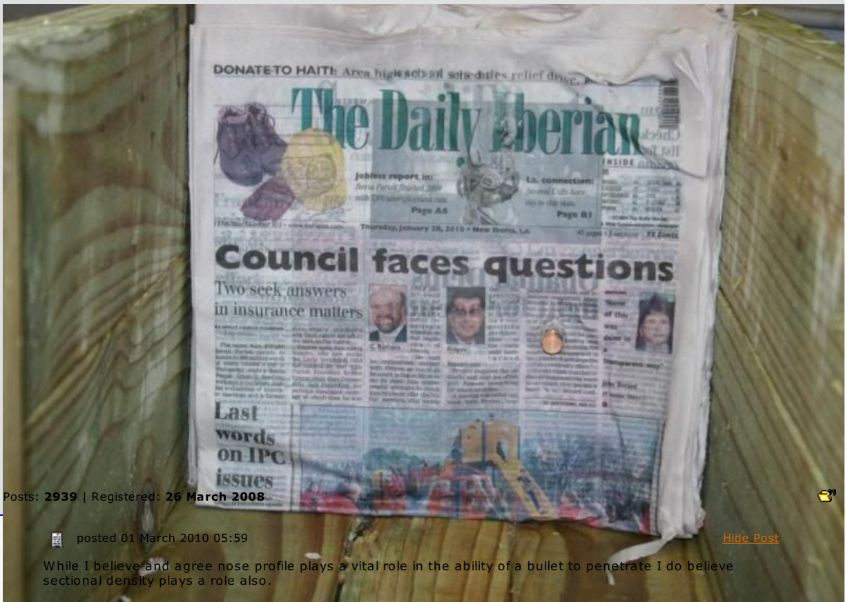
The picture above is the 11th piece of plywood the bullets penetrated. Note the location of the holes as they relate to the first picture.
