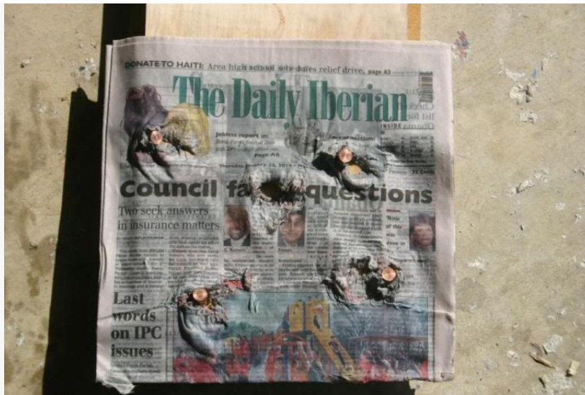
The picture is of the first piece of newspaper placed over the plywood from the back of the box. None of the bullets are more than 1" off line through 72" of penetration.
