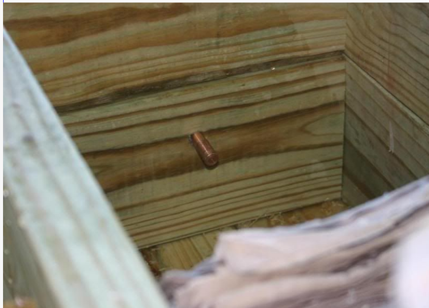
The above picture is taken from inside of box. It is another North Fork bullet after traveling through 72" of test media.
