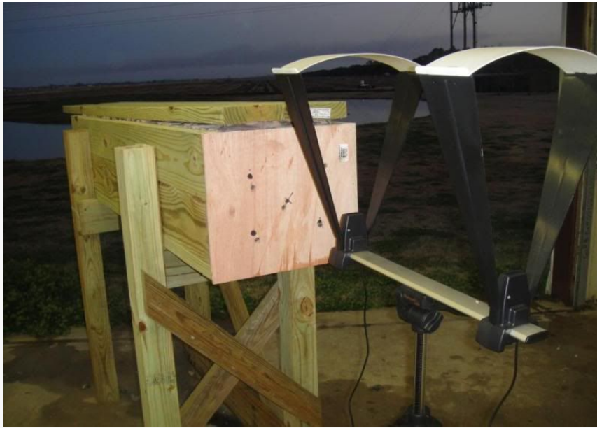
Above is the test box with chronograph.
