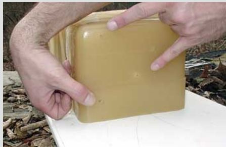
Entrance holes from handgun bullets
