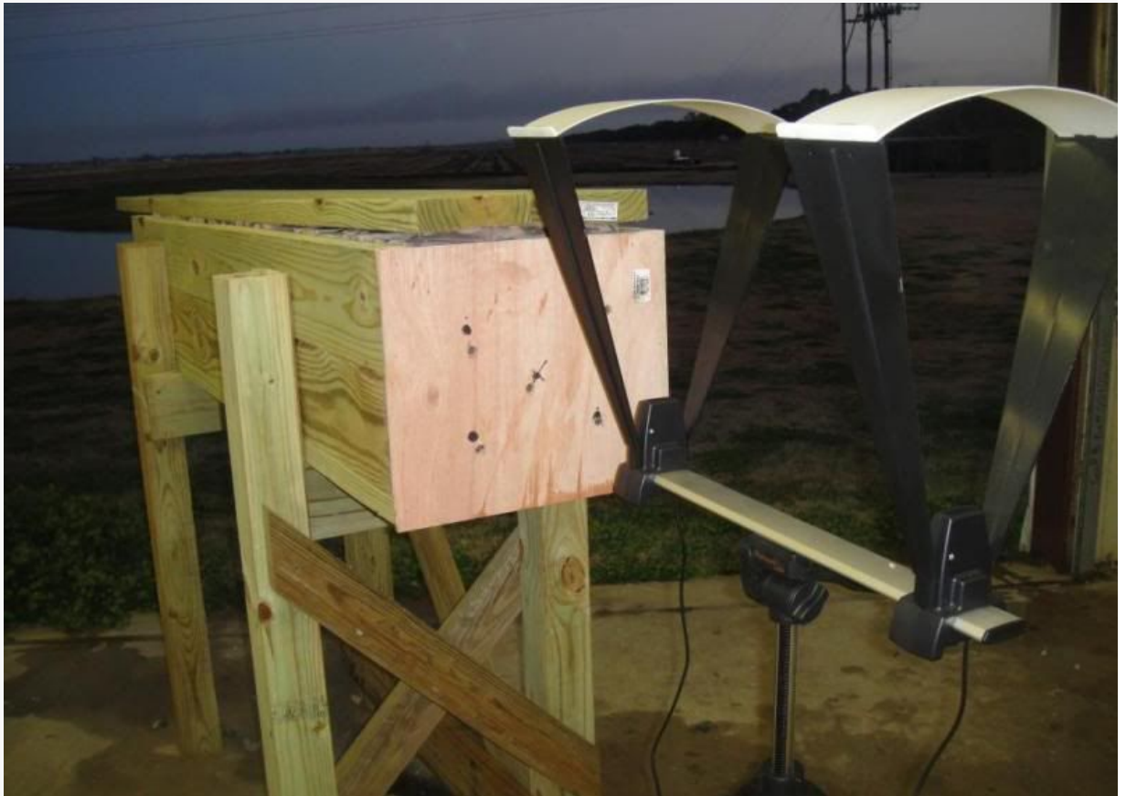
Above is the test box with chronograph.
