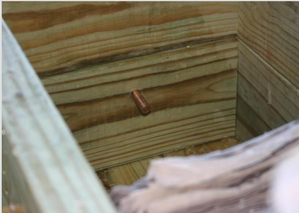
First test with 470 Nitro Northfork 72" of straight penetration. Bullet found stuck in 2 by 6 (perfectly straight).
